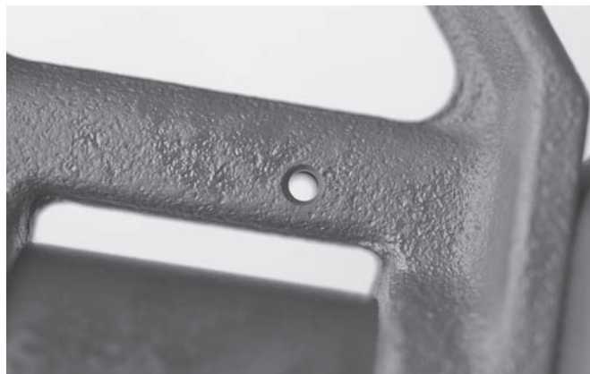
Forged front sight housings will generally have a rougher texture than cast ones.
