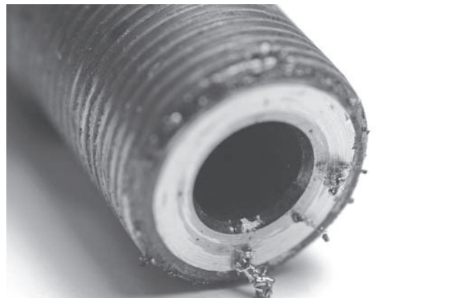
If the crown has been nicked or dented, or mis-cut from the maker, re-cutting it can improve accuracy.
