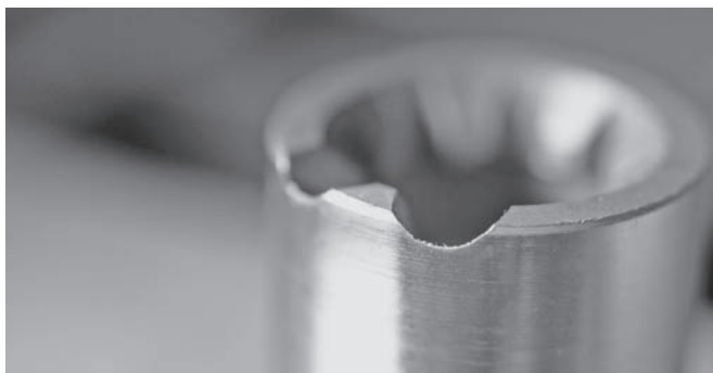
The new Colt M-4 feed ramps cut deeper into the barrel extension, and into the upper receiver.
