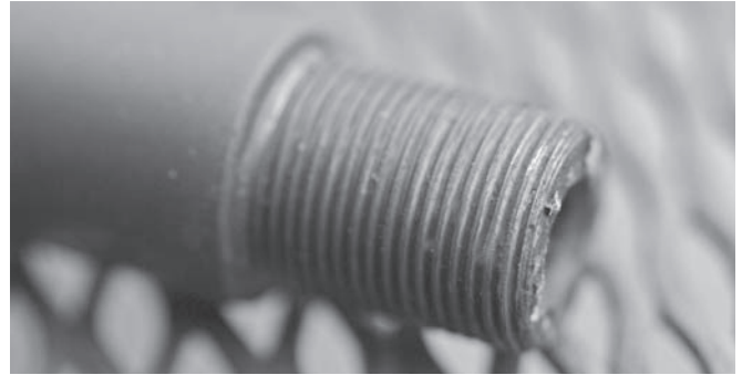
The threads allow you to attach a flash hider, which not only hides the threads, but protects the crown.
