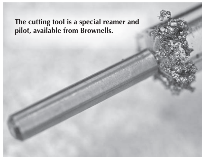
If the crown has been nicked or dented, or mis-cut from the maker, re-cutting it can improve accuracy.
