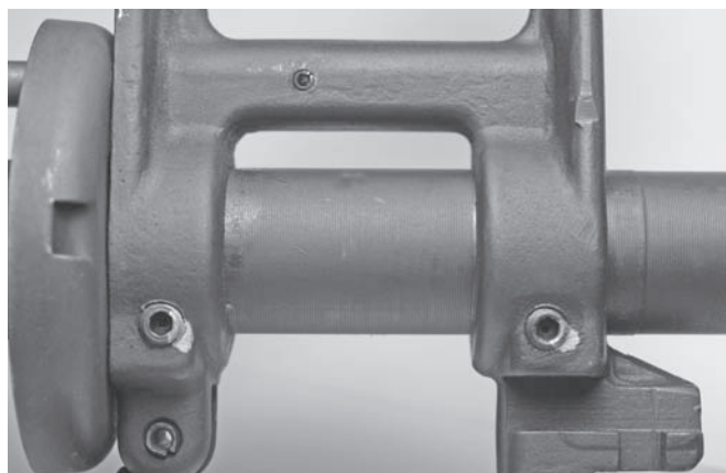
Some makers secure their front sight housings with four locking screws. The method works, but is not quite as durable as the original method.
