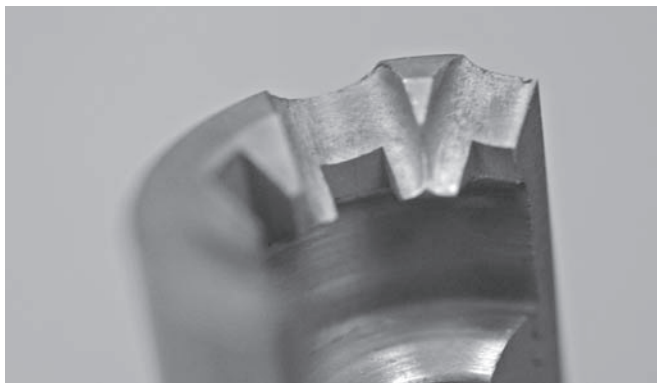
You can see the feed ramps cut on this barrel extension.
