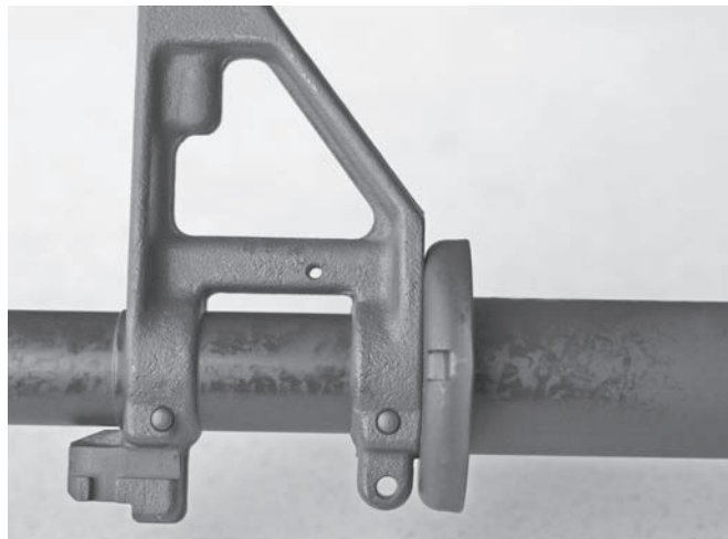
The mil-spec front sight attachment method is with a pair of taper pins.
