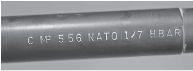
The “HBar” on this barrel means it is a heavyweight.
