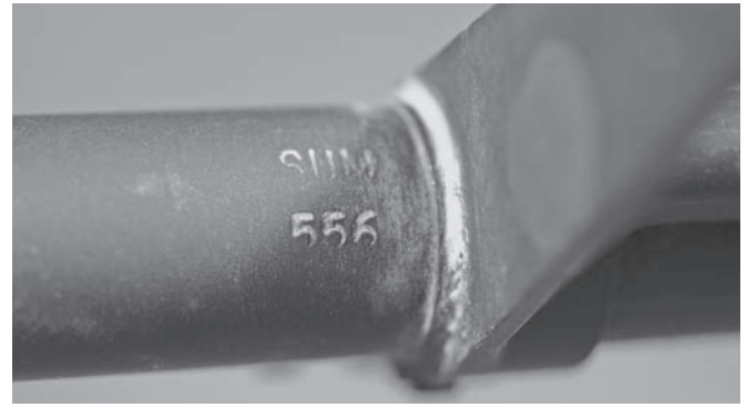
If you know the code, you know this barrel is a 5.56 chambered stainless ultra-match.
