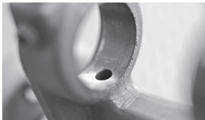
The gas gets funneled out of the port, through the front sight housing, to the gas tube and thus the carrier.
