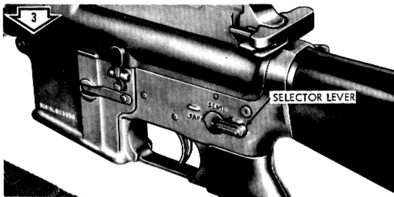
Place selector lever in SAFE position.
