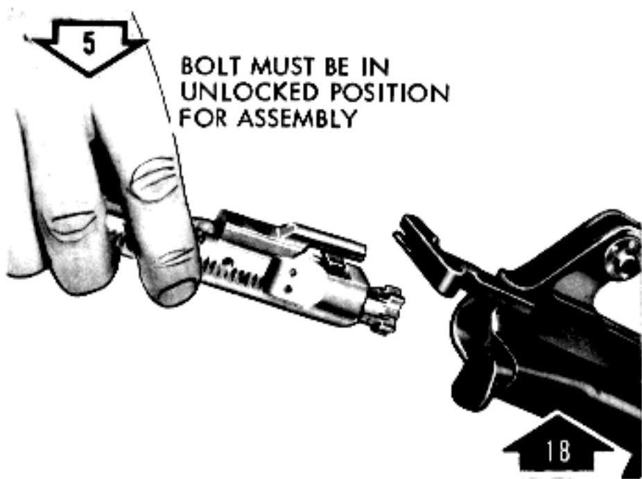
Remove/Install bolt carrier and key.
